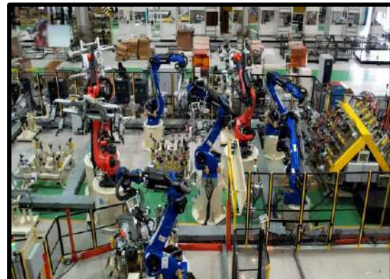
BIW Welding Line
