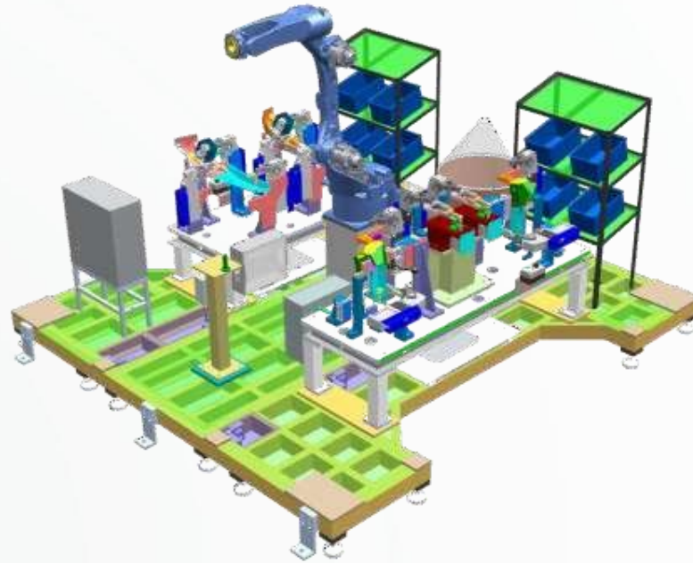
MIG Welding Fixture With Base Structure
