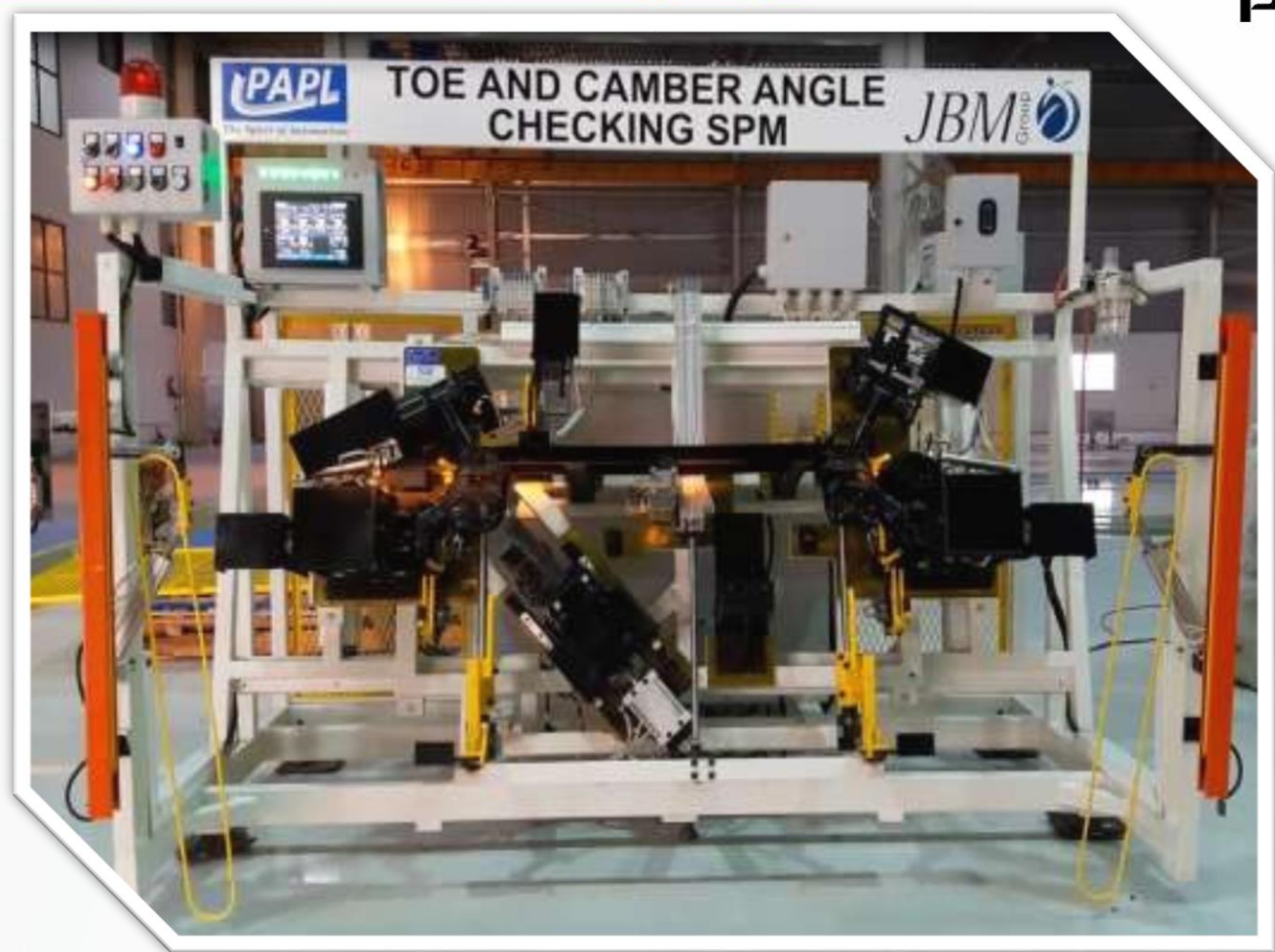
Toe and Camber Angle checking SPM
