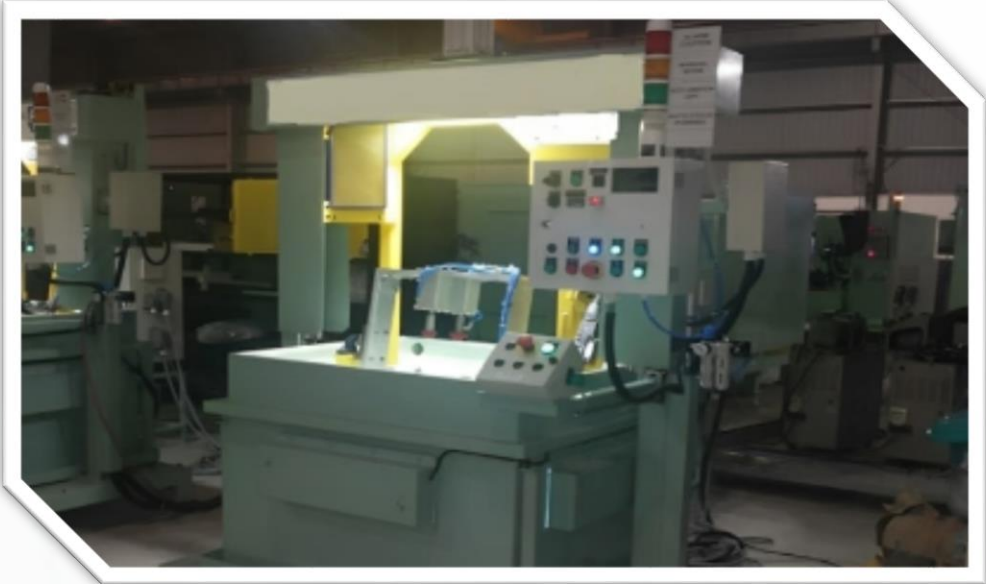
Leak Testing SPM For Fuel Tank - KWPG
