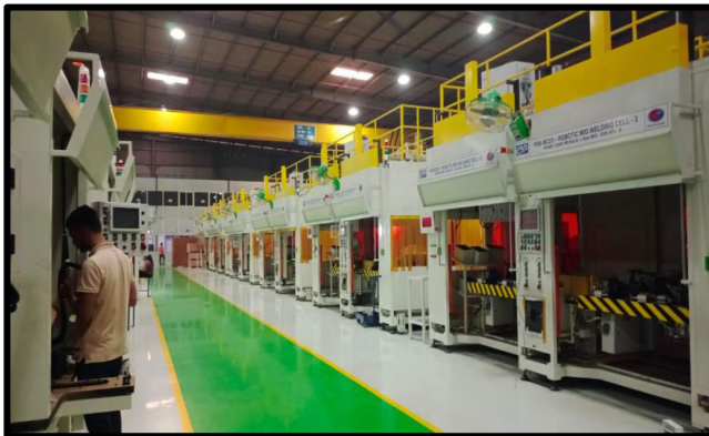
Seat Frame Welding Line
